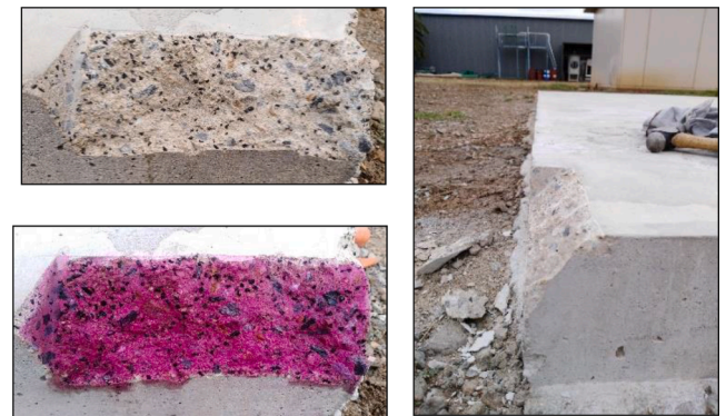
Fig. 8. Normal carbonation depth measurement.
