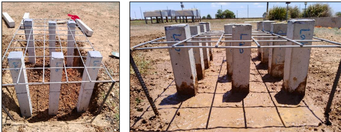
Fig. 13. Dampness and corrosion development beams buried.
