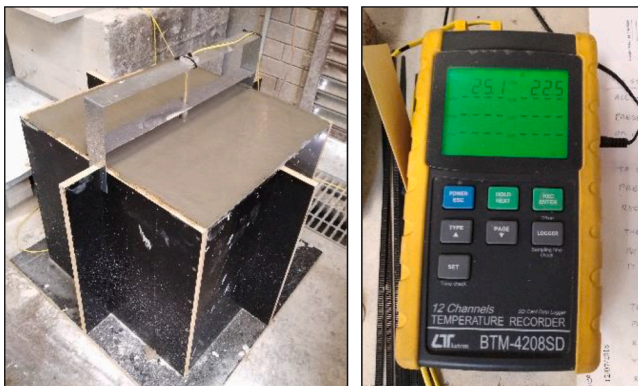
Fig. 7. Recording of hydration temperature.
