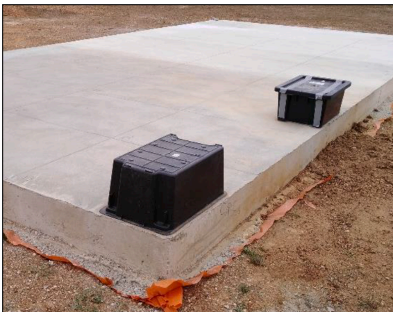
Fig. 14. Edge dampness test setup.
