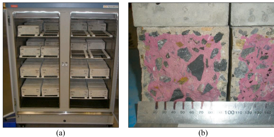
Fig. 9. Accelerated carbon dioxide ingress; (a) specimens in environmental chamber, and (b) measuring of carbonation depth.
