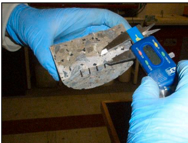
Fig. 10. Determination of the chloride ingress depth.
