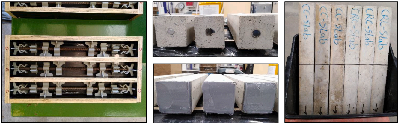
Fig. 12. Dampness and corrosion development beams and test setup.
